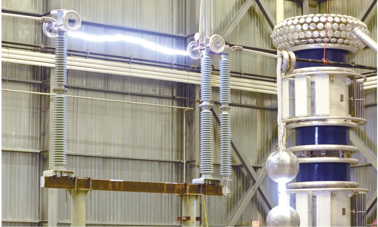
AC withstand test performed on a 362 kV AC ground switch.
